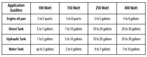
CAUTION: Do not use pads with higher than recommended wattage for specific oil capacities.
